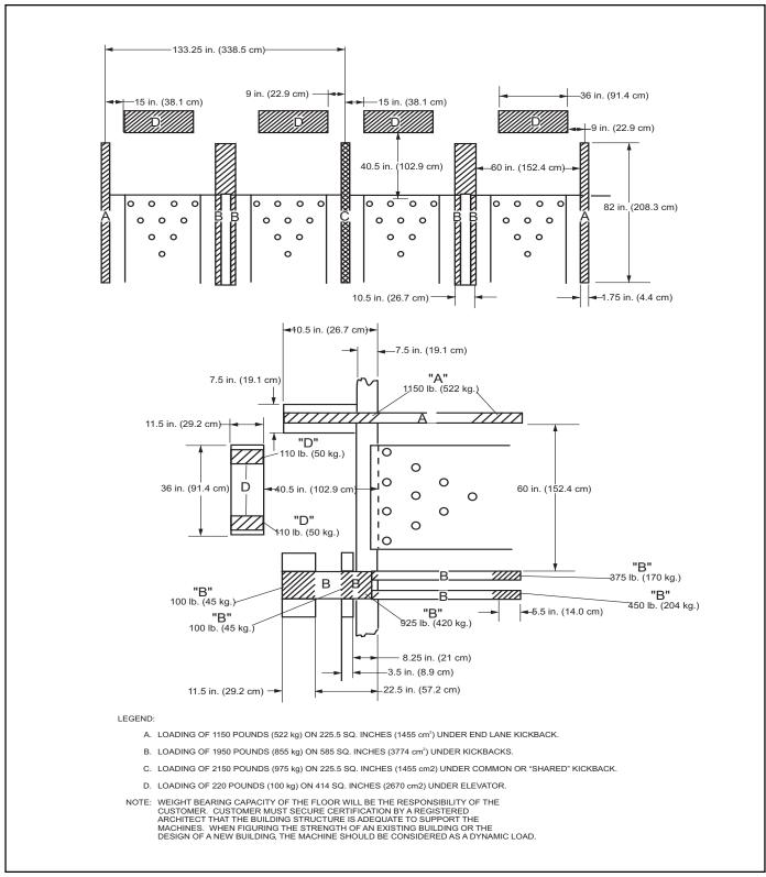
GS-Series Pinsetter Floor Loading Diagram
